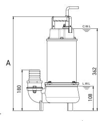
unit : mm C.W.L : Continuous running water level L.W.L : Lowest running water level
